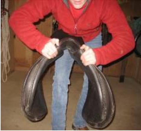
6a. To check for a broken tree down the center of the tree, press and pull on the pommel.
