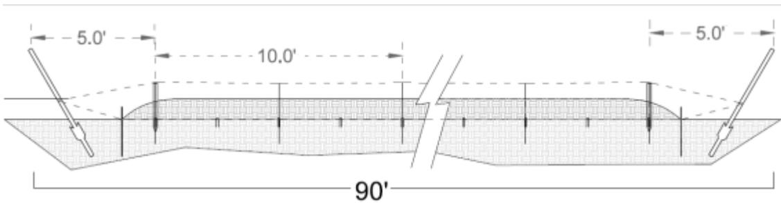
**Diagram 2.** Side view of pinned low tunnel.
