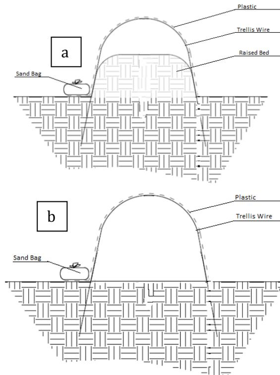
**Diagram 1.** End view of a pinned low tunnel (a) with raised bed, (b) no raised bed. Note the additional space for plants in the no raised bed option. Sand bag is for pinning the plastic down, and still allowing removal for easy ventilation.
