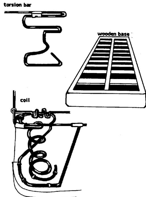
Figure 8.4. Innerspring Foundations
