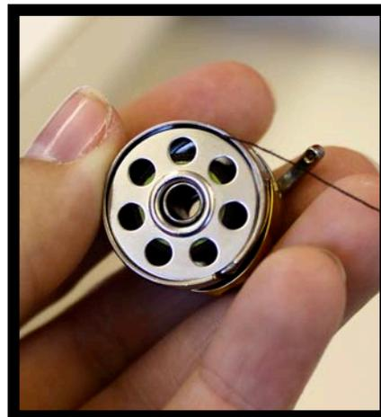
Figure 4. Bobbin case ready to install in sewing machine.
