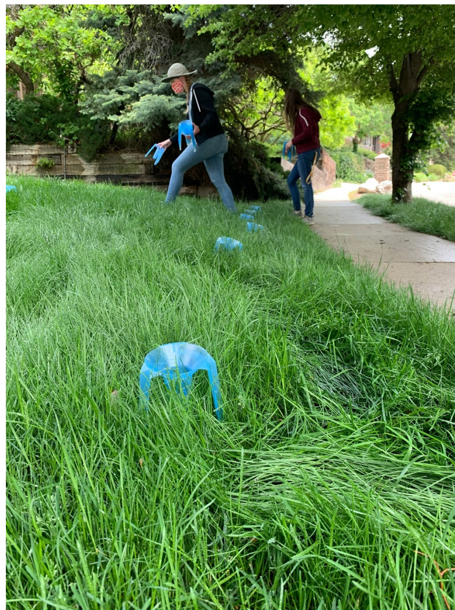
Setting up catch cups to perform a Water Check sprinkler system efficiency test (Summer, 2020).
